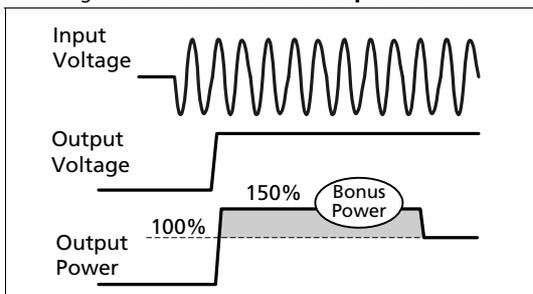
Fig. 6-8 **BonusPower<sup>®</sup> after output short**
