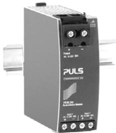
The YR80.242 is equipped with two input channels (40A each), which are individually decoupled by utilizing mosfet technology. The output current can go as high as 80A. Using mosfets instead of diodes reduces the heat generation and the voltage drop between input and output. The YR80.242 does not require an additional auxiliary voltage and is self-powered even in case of a short circuit across the output.
