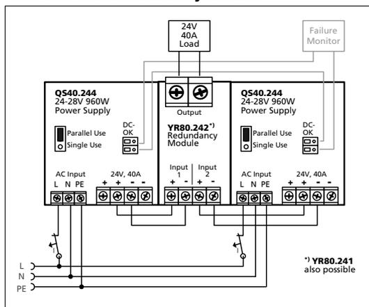
Fig. 24-2 Typical N+1 or 1+1 Redundant configuration for 40A with multiple YR40.245 redundancy modules
