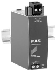
The YR40.245 is a 40A single channel redundancy module, which is equipped with a plug connector on the output. The plug connector allows replacing the power supply or the redundancy module while the system is running. The plug connector avoids that the output wires can touch and short the load circuit.
