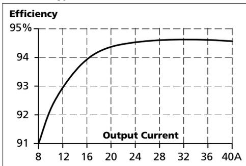
Fig. 12-2 **Losses vs. output current at 24V, typ.**
