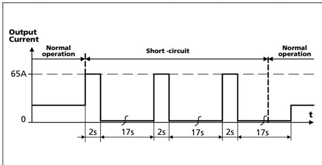
Fig. 6-4 **Dynamic overcurrent capability, typ.**
