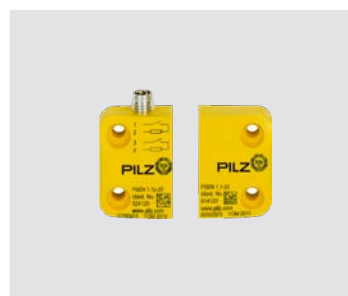
PSEN 1.1p-20/PSEN 1.1-20 Contact : 2NO Distance : 8 mm Connector : M8, 4-pin Order number : 504220
